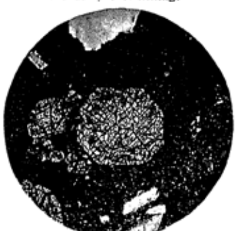
6. Enstatite, transverse section Showing form and cleavages
